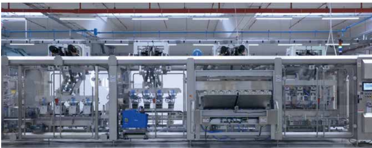
Packaging machinery by CAMA Group using two-axis robotic arms. Adopting big and fast robots requires structural rigidity obtained by steady support uprights incorporating the electrical cabinets. An example of the many unique and patented solutions developed by the Italian company.
