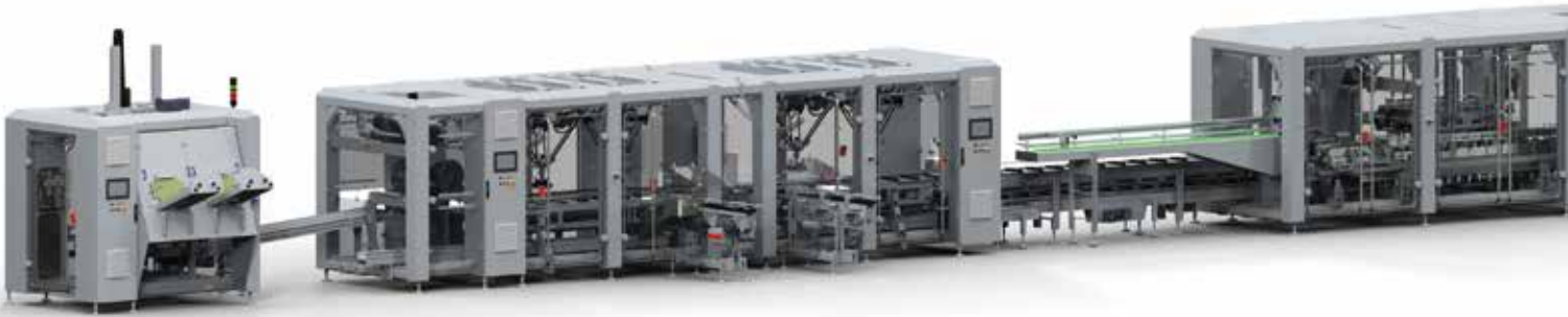
A complete packaging line developed by CAMA group for a major food company. The intensive use of robotic solutions enables the operations of several substations.
