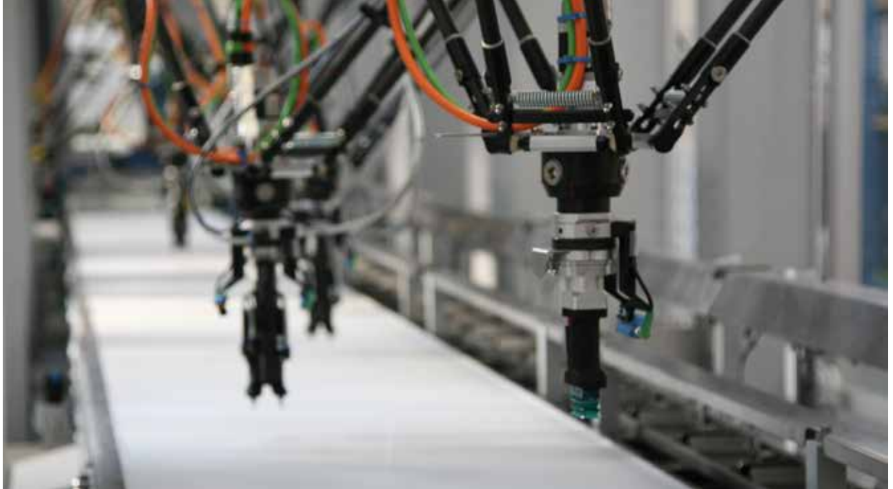
Delta robots, in detail, inside a CAMA packaging machinery.
