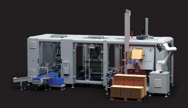
Comprising a collaborative robot, equipped with specialized gripping tools, smart cameras and advanced programming, the ACL system can automatically recognize pallet pattern, cartons stacks and interlayer sheets.
