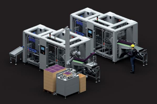
The ACL system can grip carton and case blanks and then load them into a machine's magazine automatically, removing the burden from line operators.
